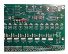
• 14 - Install three 2-pin vertical headers JP1, JP2 & JP3 (PN# 538-22-03-2021). These headers have no polarity to worry about. Install the short end through the board.
