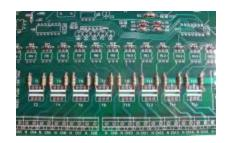
11 - Install two 0.1uF capacitors C3, C4 (PN# 80-C322C104K5R). These capacitors have no polarity to worry about.
