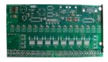
• 10 - Install 16 180 ohm resistors R26 thru R41 (PN# 291-180-RC). Make sure that the resistors have a value of 180 ohms (brown/grey/brown/gold stripes). These resistors have no polarity to worry about.
