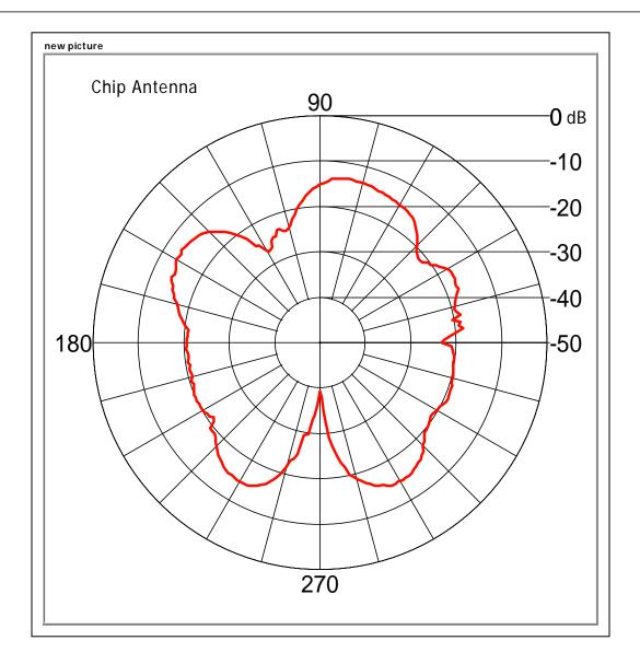
Radiation pattern of a chip antenna connected to an XBee-PRO. The pattern is normalized to the peak of the dipole antenna on the first page of this appendix, again, permitting an easy comparison.
