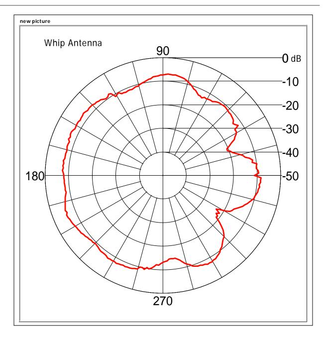
Radiation pattern of a whip antenna connected to an XBee-PRO. The pattern is normalized to the peak of the dipole antenna on the preceeding page, permitting an easy comparison.
