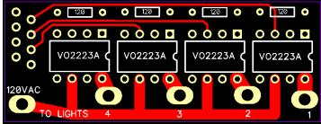
resistors should reduce the current draw for each of the VO2223A chips so that all 32 channels of the SimpleRen32 can be used simultaneously without overloading the SimpleRen32's PIC.
