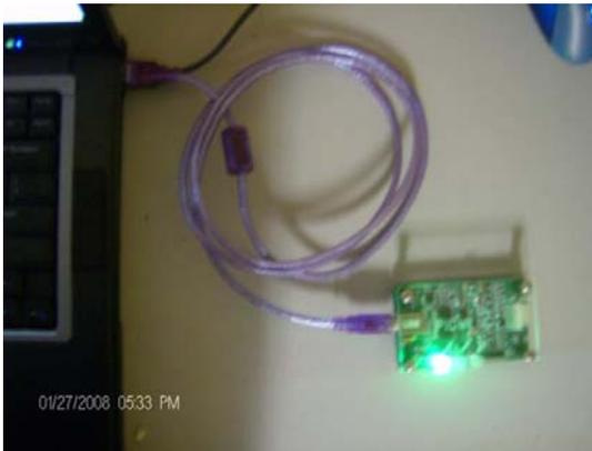
On this model you will see a green power light on the unit when it has been attached. After you attach the software may not see the programmer but have no fear you can either close and then reopen the software or click on “Tools” on the top toolbar and select “Check Communications” from the sub menu. See below pic.
