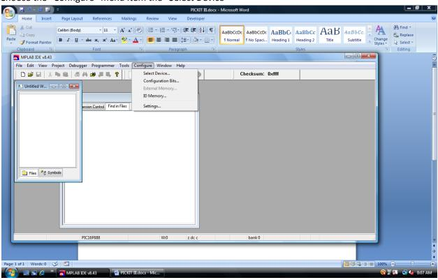
1. Choose the "PIC16F688" Chip in the device drop down
