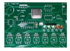
• 16 - Install the voltage regulator U1 (PN# 511-LF50CV). The voltage regulator must be installed correctly. The voltage regulators tab/heat sink must be aligned with wider line of the PCB silkscreen outline (facing towards the PCB top edge).
