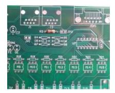
• 5 - Install two 1K ohm resistors R4, R7 (PN# 299-1K-RC). Make sure that the resistors have a value of 1K ohm (brown/black/red/gold stripes). These resistors have no polarity to worry about.
