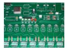
• 19 - Install four fuse clips (PN# 534-3517). Note: they are directional for proper fit of the fuse. A helpful installation tip here would be to put a fuse in the clips when you position them in their mounting holes. This will help keep them correctly aligned so that the fuse will fit properly.
