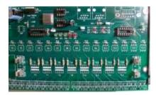
• **22** - Install 17 6-pin IC sockets for U2, M1 thru M16 (PN# 571-1-390261-1).
