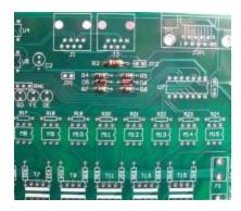
• **9** - Install 17 680 ohm resistors R6, R10 thru R25 (PN# 299-680-RC). Make sure that the resistors have a value of 680 ohms (blue/grey/brown/gold stripes). These resistors have no polarity to worry about.
