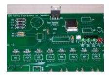
• 17 - Install the 2200uF capacitor C1 (PN# 140-REA222M1CBK1320P). This capacitor is polarized and must be installed correctly. The capacitor should have a black stripe on the body to indicate which lead is negative. The positive lead of the capacitor will be the longer lead. Make sure that the positive lead is placed in the square solder pad.
