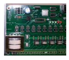
• **30** - Install two PIC microcontrollers U6 & U7 (PN# 579-PIC16F688-I/P). The PICs need to be programmed with the appropriate firmware before installation. More info on programming PICs can be found <a href="https://example.com/here.">here.</a>
