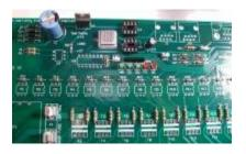
• **21** - Install two 14-pin IC sockets for U6 & U7 (PN# 571-1-390261-3).
