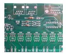
• 6 - Install three 27K ohm resistors R5, R8, R9 (PN# 299-27K-RC). Make sure that the resistors have a value of 27K ohms (red/violet/orange/gold stripes). These resistors have no polarity to worry about.
