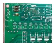
• 4 - Install the 120 ohm resistor R3 (PN# 291-120-RC). Make sure that the resistor has a value of 120 ohms (brown/red/brown/gold stripes). This resistor have no polarity to worry about.
