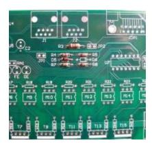
• **8** - Install zener diode D6 (PN# 78-1N5239B). The diode must be installed correctly. The diode should have a black stripe on the orange/red body. Make sure that this stripe lines up with the stripe on the PCB silkscreen (to the right).
