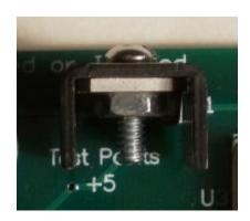
• **34** - Install two fuses (PN# 504-GMA-10) and two fuse covers (PN# 534-3527C).
