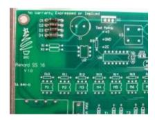
• 3 - Install two 750 ohm resistors R1 & R2 (PN# 291-750-RC). Make sure that the resistors have a value of 750 ohms (violet/green/brown/gold stripes). These resistors have no polarity to worry about.
