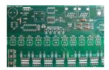
• 7 - Install zener diode D5 (PN# 78-1N5229B). The diode must be installed correctly. The diode should have a black stripe on the orange/red body. Make sure that this stripe lines up with the stripe on the PCB silkscreen (to the left).
