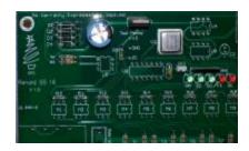
• 18 - Install the 47uF capacitor C2 (PN# 140-REA470M1CBK0511P). This capacitor is polarized and must be installed correctly. The capacitor should have a silver/grey stripe on the body to indicate which lead is negative. The positive lead of the capacitor will be the longer lead. Make sure that the positive lead is placed in the square solder pad.
